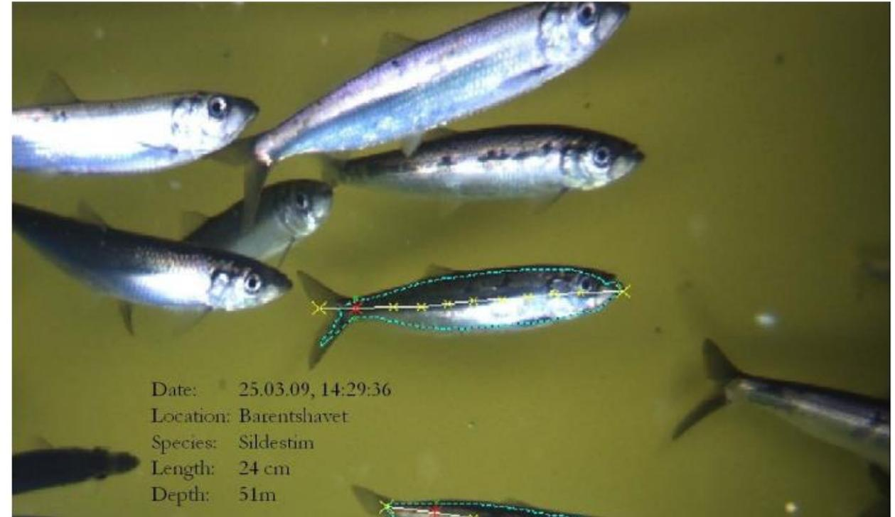
Figure 8 - Fish size and species (herring) identified in situ by stereo-optic measurements (Photo: Scantrol AS).
