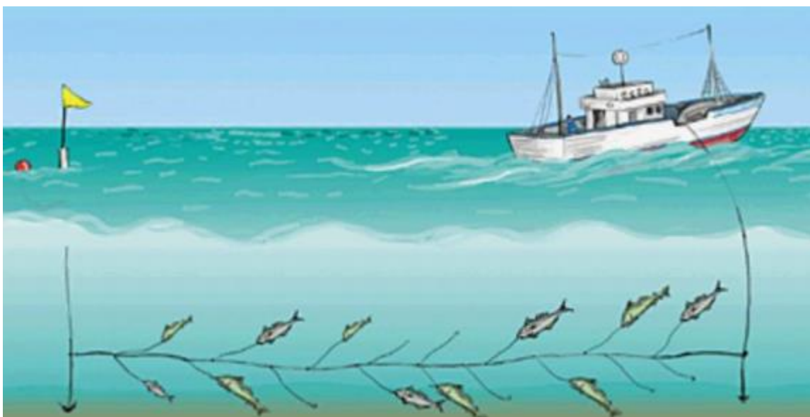
Figure 36. Fishing gear, locally known as “spinel”, used in the austral demersal fishery in the Southern Chile.
